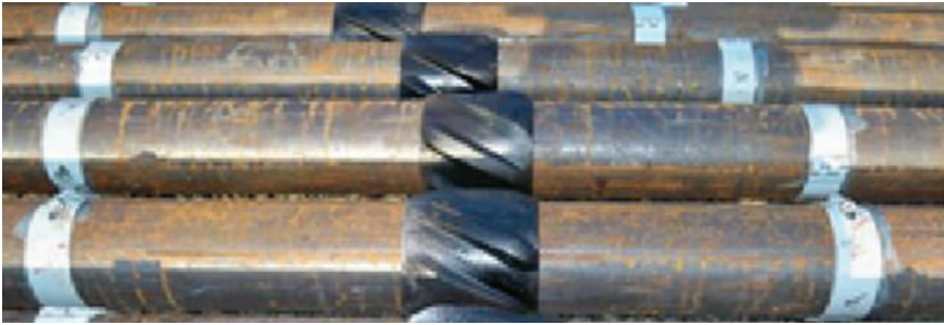
Figure 12.4: Solid body centralizers with stop collars.
