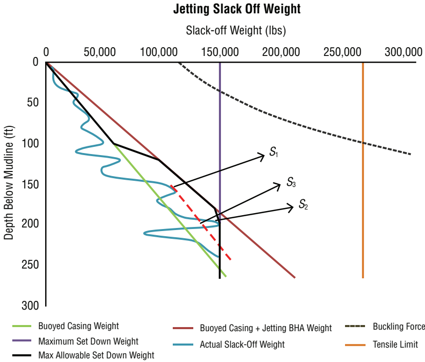
Figure 13.3: Determination of rate of strength development from plot of weight on bit while jetting.
